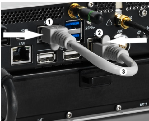
Figure 1-3: Connection between scanner unit and internal PC unit
