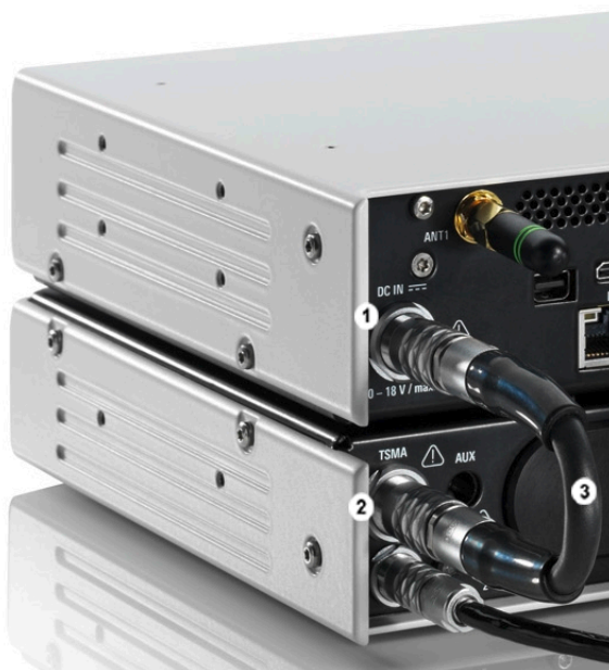
Figure 1-11: Cabling of R&S TSMA with R&S TSMA
