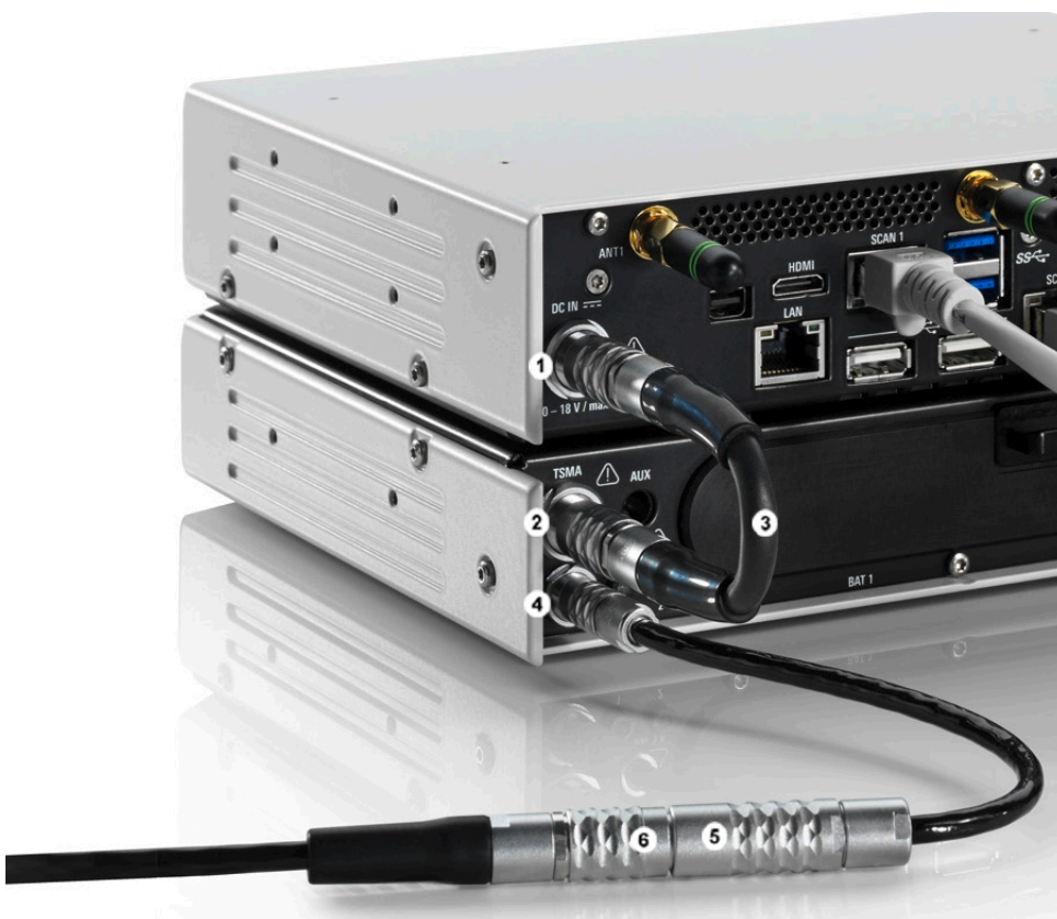
Figure 1-14: Connecting the R&S TSMA with a AC power supply
